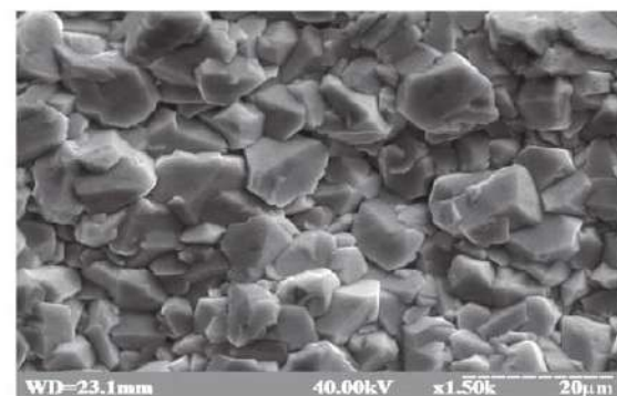
Figure 6. SEM micrographs of nondoped \text{PbO}_2 (a) \text{PbO}_2 -3.5% Nafion ® (b).
